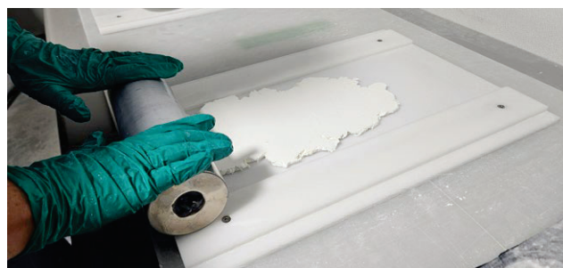
Current manufacturing processes are manual touch labor intensive, operator dependent, and susceptible to variation resulting in high scrap rates.
